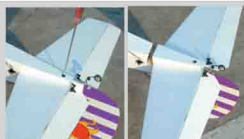
Pull-pull system for the rudder and elevator
